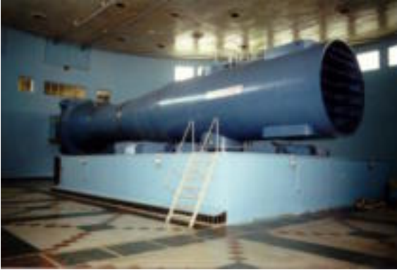
Large Centrifuge at Star City, good for 20 G's
